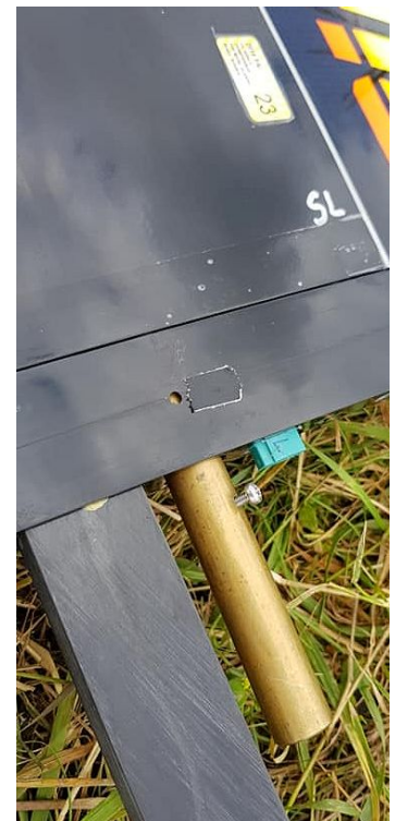
One way of installing ballast for the lightest wings without ballast tube
