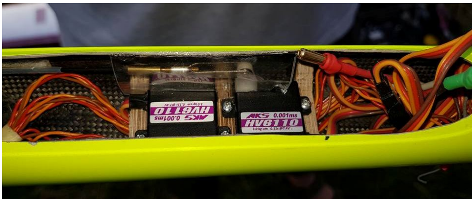
One way of installing servos in fuse for F5J version
